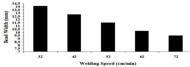
**Figure 3: Effect of Welding Speed on Weld Bead Width**
